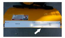
3) Cut the red dotted line off the template. Then drill a 5/16 hole.
